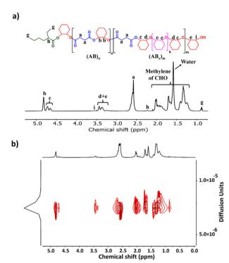
Fig. 1 (a)  $^1\text{H}$  NMR and (b) DOSY spectra (600 MHz, CDCl3, 30  $^\circ\text{C}$ ) of poly(ester-ether) (Table 1, entry 1).
