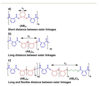
Scheme 4 Increasing distances between ester linkages in AB,  $AB_{x_r}$  and  $AB_xC$  sequences.
