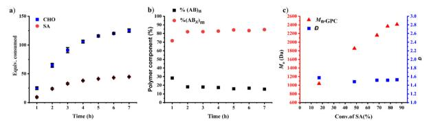
Fig. 3 ROCOP of CHO and SA using CHO: SA: SnOct<sub>2</sub> = 300:50:1 with initial [CHO]<sub>0</sub> = 2.0 M at 80 °C. (a) Plots of consumed monomers versus time, (b) plots of polymer composition versus time and (c) plots of  $M_n$  and dispersity versus conversion of SA.
