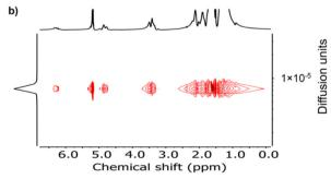
Fig. 5 (a)  $^{1}$ H NMR and (b) DOSY spectra (600 MHz, CDCl $_{3}$ , 30  $^{\circ}$ C) of poly(ester-ether)-b-PLA.
