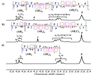
Fig. 6 <sup>1</sup>H NMR spectra (600 MHz, CDCl<sub>3</sub>, 30 °C) of (a) AB<sub>x</sub> copolymer (Table 1, entry 6, for comparison); (b)  $AB_xC$  copolymer; C = THF (Table 2, entry 4); and (c)  $AB_xC$  copolymer; C = OX (Table 2, entry 9).
