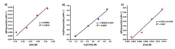
Fig. 4 Plots of initial rates versus (a) SA concentration, (b) CHO concentration and (c) SnOct<sub>2</sub> concentration.
