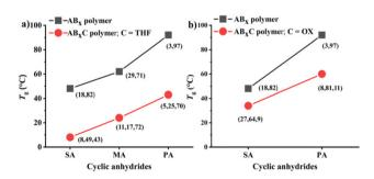
Fig. 8 Comparison of glass-transition temperatures  $(T_q)$  between  $AB_x$ and  $AB_xC$  polymers where (a) C = THF and (b) C = OX, given that (X,Y) =%AB and %AB<sub>x</sub>, respectively, and (X,Y,Z) = %AB, %AB<sub>x</sub> and %AB<sub>x</sub>C, respectively.
