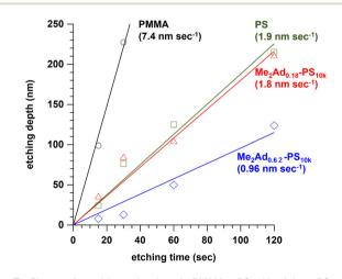
Fig. 7 Plots of etching depth of PMMA, PS, Me<sub>2</sub>Ad<sub>0.18</sub>-PS and Me<sub>2</sub>Ad<sub>0.62</sub>-PS thin films with increasing etching time. The values in parentheses represent the etching rate determined by the slope.
