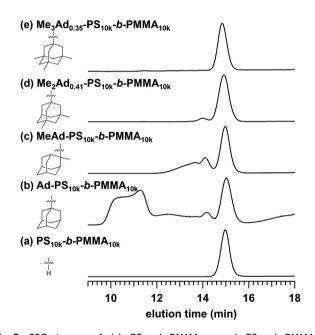
Fig. 2 SEC traces of (a)  $PS_{10k}$ -b- $PMMA_{10k}$  and  $PS_{10k}$ -b- $PMMA_{10k}$  modified with (b) Ad-OH, (c) MeAd-OH, (d) Me<sub>2</sub>Ad-OH, and (e) Me<sub>3</sub>Ad-OH ([styrene unit]<sub>0</sub>/[adamantanol]<sub>0</sub>/[TfOH] = 1.00/0.50/0.75).
