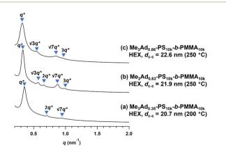
Fig. 10 SAXS profiles of the thermally annealed Me<sub>3</sub>Ad-PS<sub>10k</sub>-b- $PMMA_{10k}$ . (a)  $Me_3Ad_{0.35}-PS_{10k}-b-PMMA_{10k}$ , (b)  $Me_3Ad_{0.63}-PS_{10k}-b-PMMA_{10k}$ PMMA<sub>10k</sub> and (c) Me<sub>3</sub>Ad<sub>0.86</sub>-PS<sub>10k</sub>-b-PMMA<sub>10k</sub>. The value in the parentheses represents the annealing temperature.
