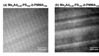
Fig. 9 TEM micrographs of (a)  $Me_2Ad_{0.29}$ - $PS_{10k}$ -b- $PMMA_{10k}$  (annealed at 200 °C for 24 h) and (b)  $Me_2Ad_{0.28}$ - $PS_{14k}$ -b- $PMMA_{14k}$  (annealed at 250 °C for 24 h).
