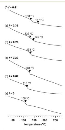
Fig. 6 Second heating DSC traces of (a) PS<sub>10k</sub>-b-PMMA<sub>10k</sub>,  $Me_2Ad_{0.07}$ - $PS_{10k}$ -b- $PMMA_{10k}$ , (c)  $Me_2Ad_{0.20}-PS_{10k}-b-PMMA_{10k}$ ,  $Me_2Ad_{0.29}-PS_{10k}-b-PMMA_{10k}$ (e)  $Me_2Ad_{0.38}-PS_{10k}-b-PMMA_{10k}$  and (f) Me<sub>2</sub>Ad<sub>0.41</sub>-PS<sub>10k</sub>-b-PMMA<sub>10k</sub>.
