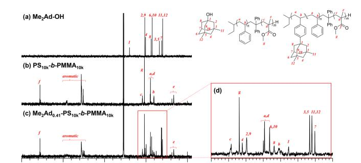
Fig. 3  $^{13}$ C NMR spectra of (a) Me<sub>2</sub>Ad-OH and (b) PS<sub>10k</sub>-b-PMMA<sub>10k</sub> in CDCl<sub>3</sub> (100 MHz), and (c) inverse-gated decoupling  $^{13}$ C NMR spectrum of Me<sub>2</sub>Ad<sub>0.41</sub>-PS<sub>10k</sub>-b-PMMA<sub>10k</sub> (lower) in CDCl<sub>3</sub> (100 MHz). (d) The expansion from 60 to 25 ppm of the spectrum (c).
