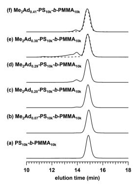
Fig. 5 SEC traces of  $Me_2Ad-PS_{10k}-b-PMMA_{10k}$  samples (b)–(f) and the corresponding  $PS_{10k}-b-PMMA_{10k}$  (a) (eluent, THF; flow rate, 1.0 mL min<sup>-1</sup>). The dashed curves represent the SEC traces after preparative SEC purification.
