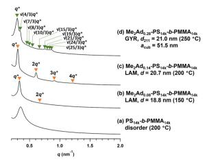
Fig. 11 SAXS profiles of the thermally annealed Me<sub>2</sub>Ad-PS<sub>14k</sub>-b- $PMMA_{14k}$ . (a)  $PS_{14k}-b-PMMA_{14k}$ , (b)  $Me_2Ad_{0.08}-PS_{14k}-b-PMMA_{14k}$ , (c)  $Me_2Ad_{0.14}-PS_{14k}-b-PMMA_{14k}$  and (d)  $Me_2Ad_{0.28}-PS_{14k}-b-PMMA_{14k}$ . The value in the parentheses represents the annealing temperature.
