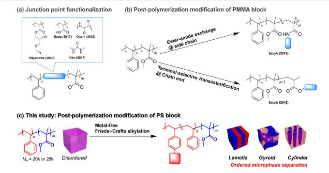
Fig. 1 Chemical modification of PS-b-PMMA. (a) Previous works on the junction point functionalization. (b) Previous works on the PMMA side-chain and chain-end functionalization via post-polymerization modification of commercially available PS-b-PMMA. (c) This work, which focuses on post-polymerization modification of the PS block via the metal-free Friedel–Crafts alkylation reaction.
