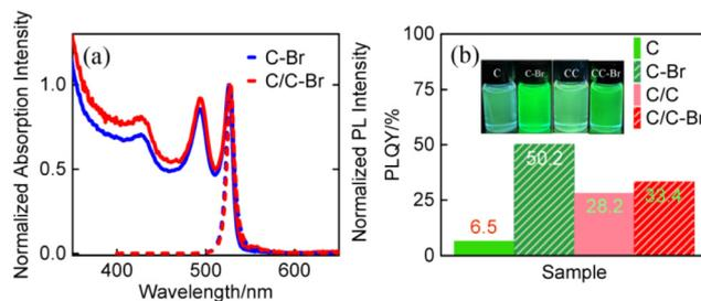
**Fig. 5** (a) Normalized absorption and PL spectra of C and C/C NPLs after 5 h of ligand exchange. (b) PLQYs before and after ligand exchange for C and C/C NPLs. Insets: images of the samples before and after ligand exchange under UV light illumination.
