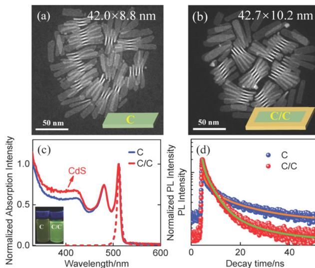
**Fig. 1** STEM image of (a) C, (b) C/C NPLs. Insets are the schematic diagrams of their corresponding structures. (c) Normalized UV-visible absorption and PL spectra of C and C/C NPLs. Inset is the image of samples under UV light illumination. (d) Room temperature TRPL of C and C/C NPLs.
