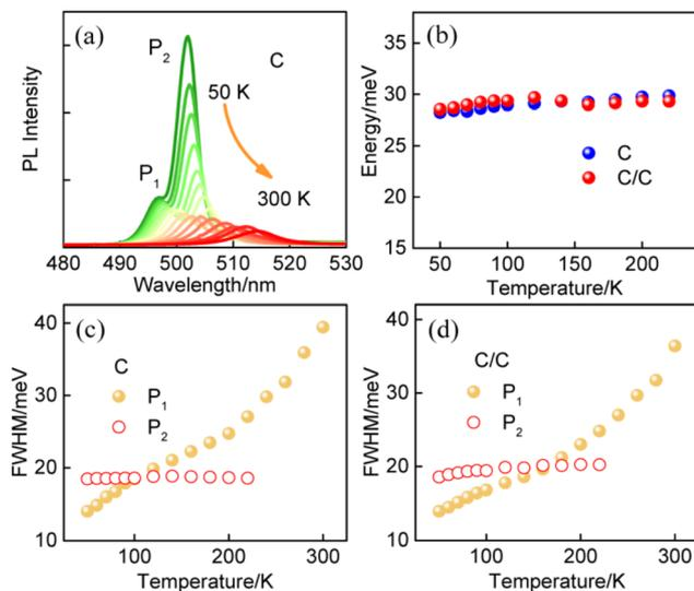
**Fig. 2** (a) Temperature-dependent PL spectra of C NPLs. (b) Energy difference of  $P_1$  and  $P_2$  of C and C/C NPLs. (c) FWHM of the  $P_1$  and  $P_2$  of C NPLs at different temperatures. (d) FWHM of the  $P_1$  and  $P_2$  of C/C NPLs at different temperatures.
