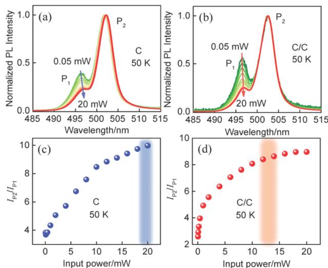
**Fig. 3** Power-dependent PL spectra of (a) C and (b) C/C NPLs at 50 K. (c) C and (d) C/C NPLs Power-dependent ratio of  $P_2/P_1$ . The cylinders represent the initial saturation power of C and C/C NPLs, respectively.
