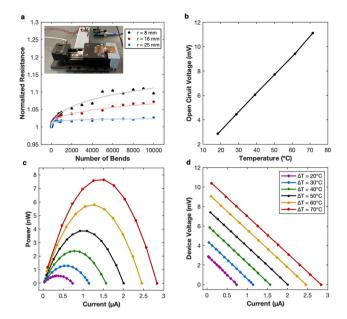
Fig. 5 Electrical characterization of single leg TE film sintered at 425 °C. (a) Resistance as a function of bending cycles for various radii of curvature. Inset shows bending test apparatus. (b) Open circuit voltage as a function of temperature difference, (c) device voltage as a function of current and (d) power curves for several temperature differentials.
