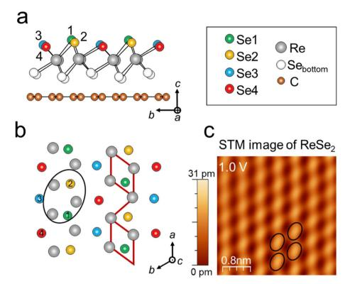
Fig. 1 Monolayer (ML) ReSe<sub>2</sub> on a graphene substrate. (a and b) The side- and top-view structures of ML ReSe<sub>2</sub>. The Se atoms in the topmost layer are classified into Se1 (green), Se2 (orange), Se3 (blue), and Se4 (red) based on their height along the c-axis. The Re-chain is indicated by red solid lines in (b). (c) The STM topography image of ReSe<sub>2</sub> shows the oval feature with a lattice constant of  $\sim$ 6.6 Å ( $I_t = 30$  pA).
