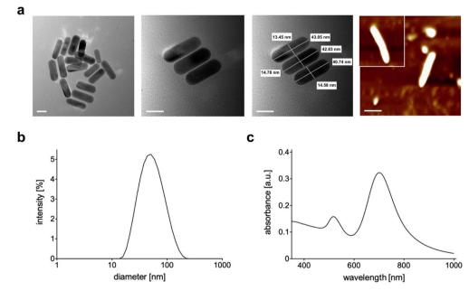
Fig. 2 (a) TEM and AFM (last panel) images of Au NRs (scale bar = 20 nm); (b) DLS analysis of Au NRs; (c) absorption spectrum of Au NRs.
