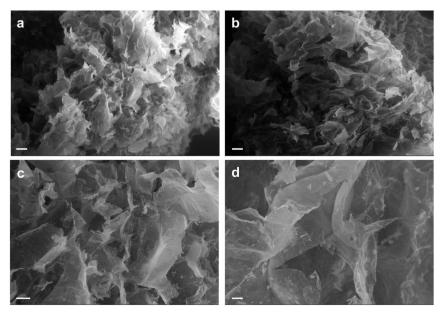
Fig. 4 SEM analysis of AC hydrogels loaded with Au NRs (a and c) and neat AC hydrogels (b and d). Scale bars: 200 µm (a and b); 100 µm (c and d).
