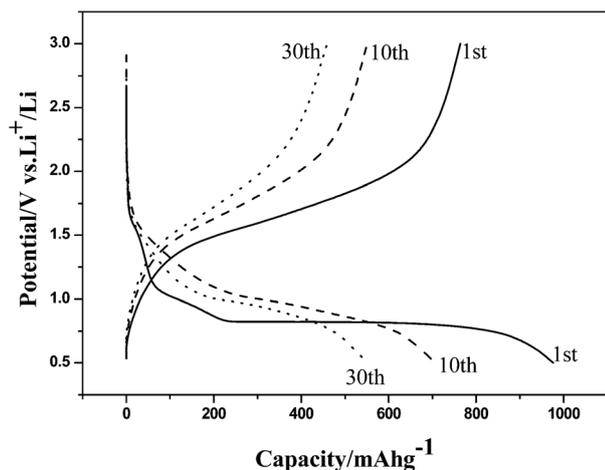
Fig. 19 The first (solid line), 10th (dashed line), and 30th (dotted line) charge–discharge curves of flower-like  $\alpha$ - $\text{Fe}_2\text{O}_3$  nanostructures at a current density of  $0.2 \text{ mA cm}^{-2}$ . Reprinted with permission from ref. 306. Copyright © 2008, American Chemical Society. All rights reserved.
