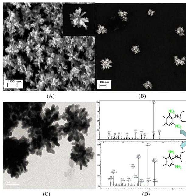
Fig. 6 (A and B) SEM and (C) TEM images of gold nanoflowers that are synthesized; mass spectral data of (D) show the process of degradation of pendimethalin (above) to *N*-(1-ethylpropyl)-2,6-diamino-3,4-xylidine (below). Reprinted with permission from ref. 139. Copyright © 2014, American Chemical Society. All rights reserved.
