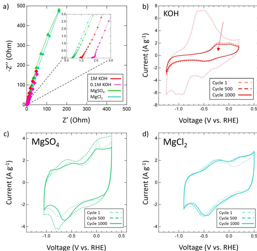
Fig. 6 (a) EIS spectra for 1 M KOH (red), 0.1 M KOH (pink), 1 M MgSO<sub>4</sub> (green) and 1 M MgCl<sub>2</sub> (cyan) with a frequency range of 200 kHz to 10 mHz and an amplitude of 10 mV; (b) stability CVs of VN in (b) 1 M KOH, (c) MgSO<sub>4</sub> and (d) MgCl<sub>2</sub> at 50 mV s<sup>-1</sup> at cycle 1, cycle 500, and cycle 1000.
