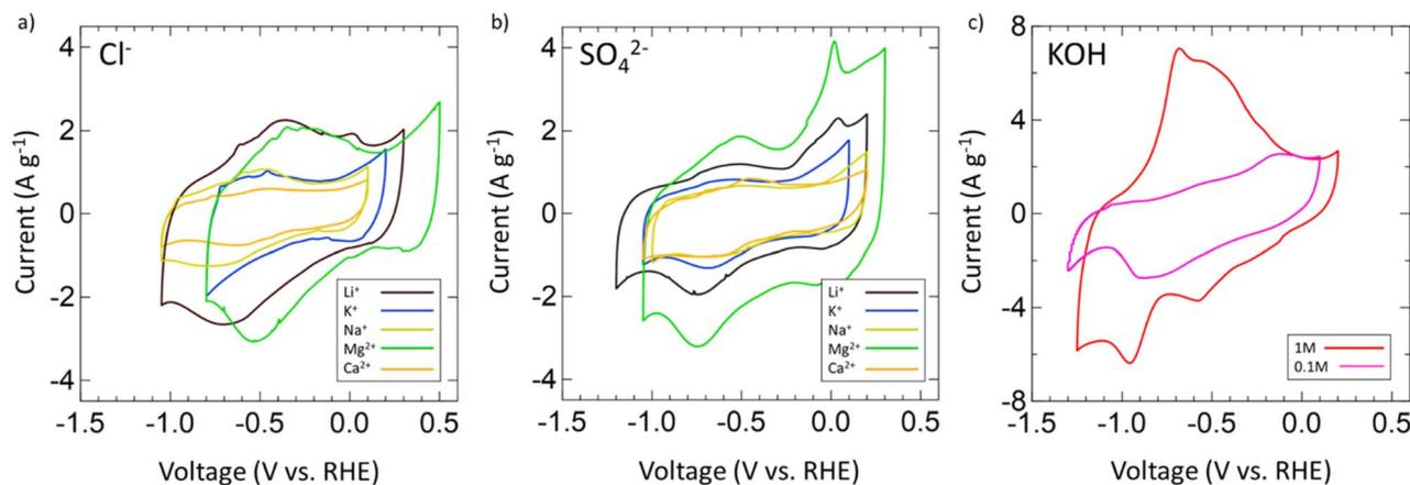
Fig. 3 CVs of operating voltage windows for (a) chlorides, (b) sulfates of  $\text{Mg}^{2+}$  (green),  $\text{Li}^+$  (black),  $\text{K}^+$  (blue),  $\text{Na}^+$  (yellow), and  $\text{Ca}^{2+}$  (orange) at  $50 \text{ mV s}^{-1}$ . (c) CVs for 1 M (red) and 0.1 M (pink) KOH. All chlorides and sulfates are 1 M concentration except for  $\text{K}_2\text{SO}_4$  (0.5 M),  $\text{CaSO}_4$  (0.06 M), and  $\text{CaCl}_2$  (0.02 M) due to low solubility at room temperature.
