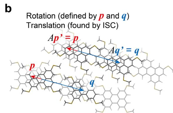
Fig. 4 Construction of the neighboring layer in the iBW structure of MT-perylene from the BW structure. The mirror plane can be chosen arbitrarily and is  $y = 8.5 \text{ \AA}$  in the present case (a). Rotation matrix  $A$  in (b) is defined in eqn (1) to ensure  $A\mathbf{q}' = \mathbf{q}$  (and  $A\mathbf{p}' = \mathbf{p}$ ).
