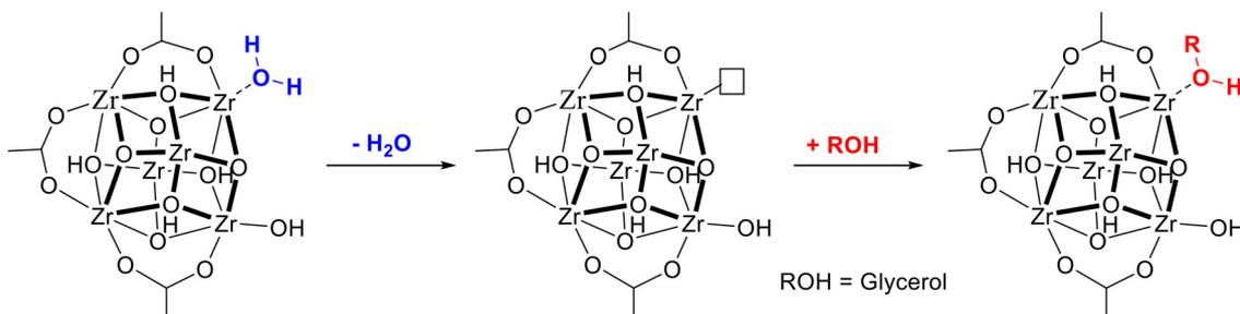
Fig. 5 Removal of polarized H<sub>2</sub>O molecules during UiO-66 dehydration and formation of novel Brønsted-induced acid sites upon glycerol adsorption.
