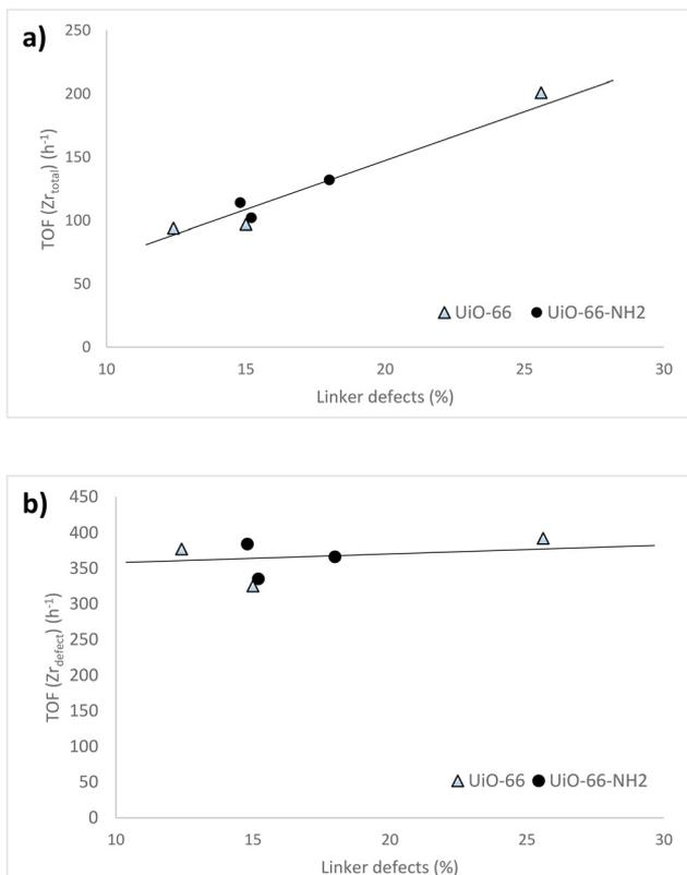
**Fig. 6** a) TOF ( $Zr_{total}$ ) & linker defect and b) TOF ( $Zr_{defect}$ ) & linker defect plots for the acetalization reaction of phenylacetaldehyde with glycerol in the presence of UiO-66 and UiO-66-NH<sub>2</sub> catalysts. Reaction conditions: PhA (2 mmol), glycerol (4 mmol), MOF 10 mg (ca. 1.5 mol% Zr), reflux of toluene (6 mL), Dean-Stark.
