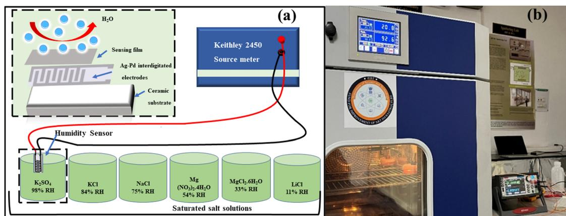
**Fig. 1** (a) An illustration depicting the arrangement of the humidity-sensing setup, which includes various saturated salt solutions with distinct humidity levels, as well as the source meter; (b) cabinet for controlling temperature and humidity to maintain precise and stable temperature and humidity conditions.
