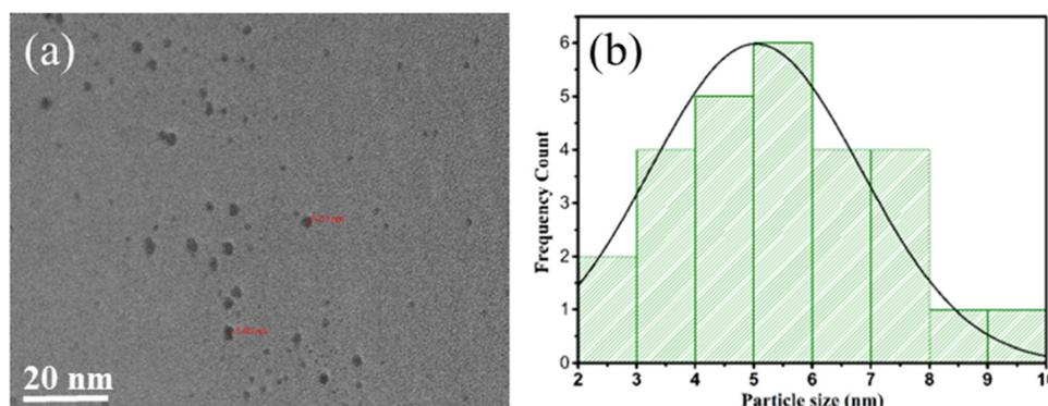
Fig. 7 (a) HRTEM image; (b) histogram for the particle size distribution of 6%-WO<sub>3</sub>/COK-12.
