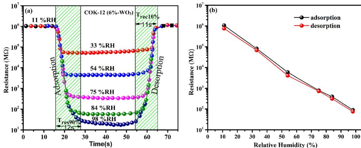
Fig. 10 (a) Response/recovery curve across diverse humidity levels for the 6%-WO<sub>3</sub>/COK-12 configuration; (b) Hysteresis curve displaying the lag between the adsorption and desorption process of the sensor.
