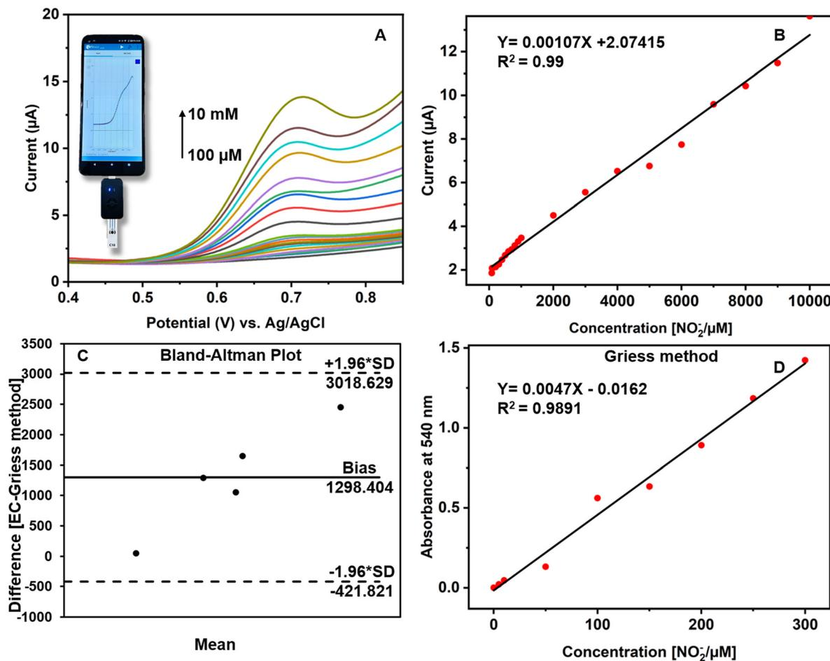
Fig. 5 (A) LSV response of the CuCP-MWCNTs-SPCE towards various concentrations of nitrite ranging from 100  $\mu\text{M}$  to 10 mM. Calibration plot of the CuCP-MWCNTs-SPCE towards nitrite detection in human saliva samples (B). Comparison of the electrochemical and Griess method results using a Bland-Altman plot (C). Calibration plot of the Griess method towards nitrite detection in human saliva samples (D).
