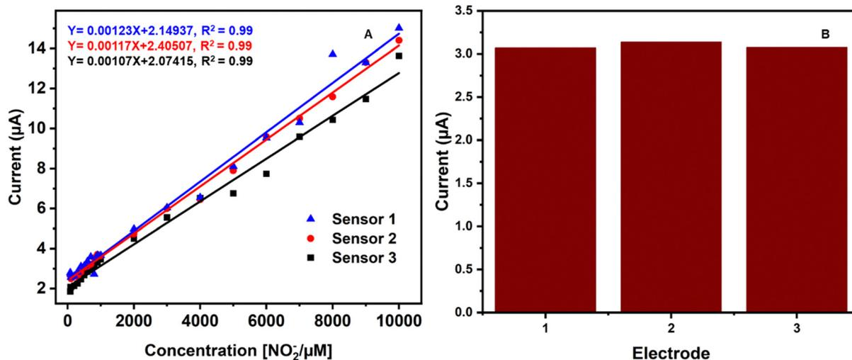
Fig. 6 Reproducibility investigation of CuCP-MWCNTs-SPCE towards nitrite detection with the (a) calibration curves for the concentration between 100  $\mu\text{M}$  and 10 mM; (b) intra-study of three sensors in 500  $\mu\text{M}$  nitrite in saliva samples with 0.01 M PBS.
