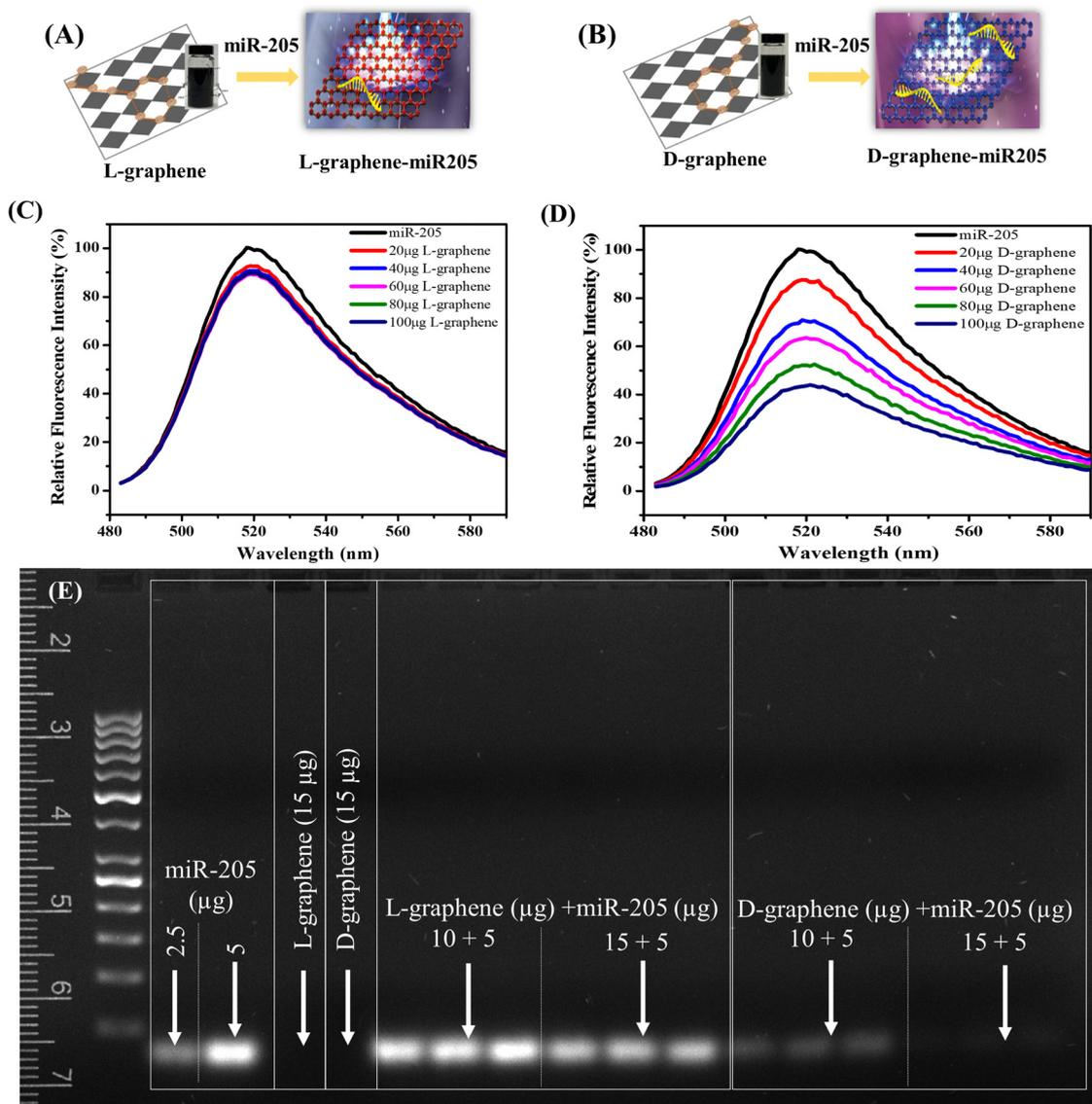
**Fig. 4** D-Graphene promotes superior complexation with miR-205. (A–B) Schematic representation of L-graphene and D-graphene complexation with miR-205. Nano complexation study of miR-205 through fluorescence-based binding and quenching methods. Fluorescence spectra of (C) L-graphene and (D) D-graphene with fluorescein amidite (FAM)-labelled miRNA (FAM-miR-205). (E) Nano complexation study of miR-205 with L-graphene and D-graphene through 2D-agarose gel electrophoresis.
