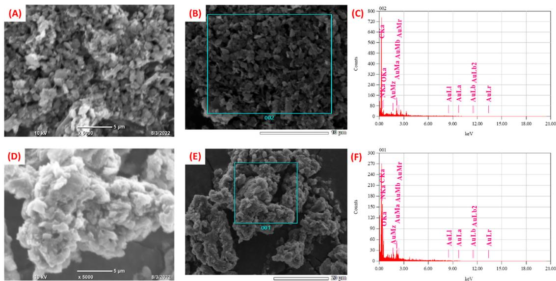
Fig. 3 SEM images of (A) and (B)  $C_3N_4$ /RGO and (D) and (E) bio-functionalized  $C_3N_4$ /RGO nanocomposite. Elemental distribution of (C)  $C_3N_4$ /RGO and (F) bio-functionalized  $C_3N_4$ /RGO nanocomposite respectively.
