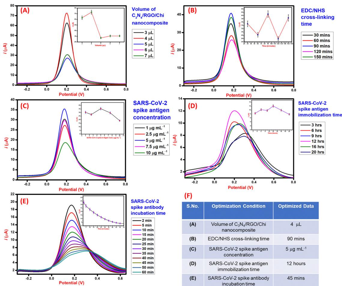
Fig. 5 The optimization data for the fabrication of the immunosensor; (A) volume of  $C_3N_4$ /RGO/Chi nanocomposite, (B) EDC/NHS cross-linker incubation time, (C) SARS-CoV-2 spike antigen concentration, (D) SARS-CoV-2 spike antigen immobilization time, and (E) SARS-CoV-2 antibody incubation time, 0.1 M PBS (pH 7.4) containing 0.1M KCl and 5 mM ferri/ferrocyanide redox solution, (F) the summarized optimization data in tabular format.
