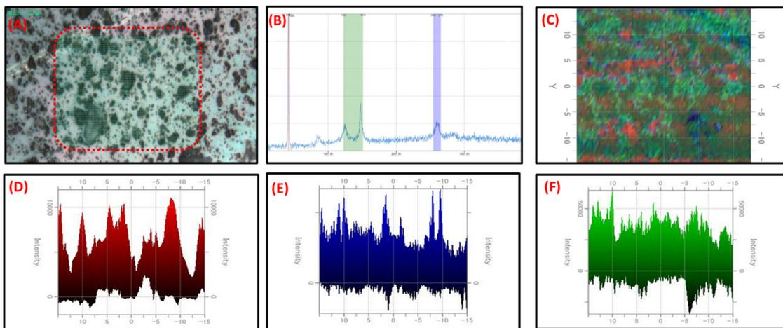
Fig. 2 (A) Optical image bio-functionalized  $C_3N_4$ /RGO nanocomposite on silica substrate at  $100\times$  magnification, (B) Raman spectra of bio-functionalized  $C_3N_4$ /RGO nanocomposite on a silica substrate, (C) Raman mapping image of the bio-functionalized  $C_3N_4$ /RGO nanocomposite, 2D Raman mapping image of (D) Si, (E) Chi, (F)  $C_3N_4$ /RGO.
