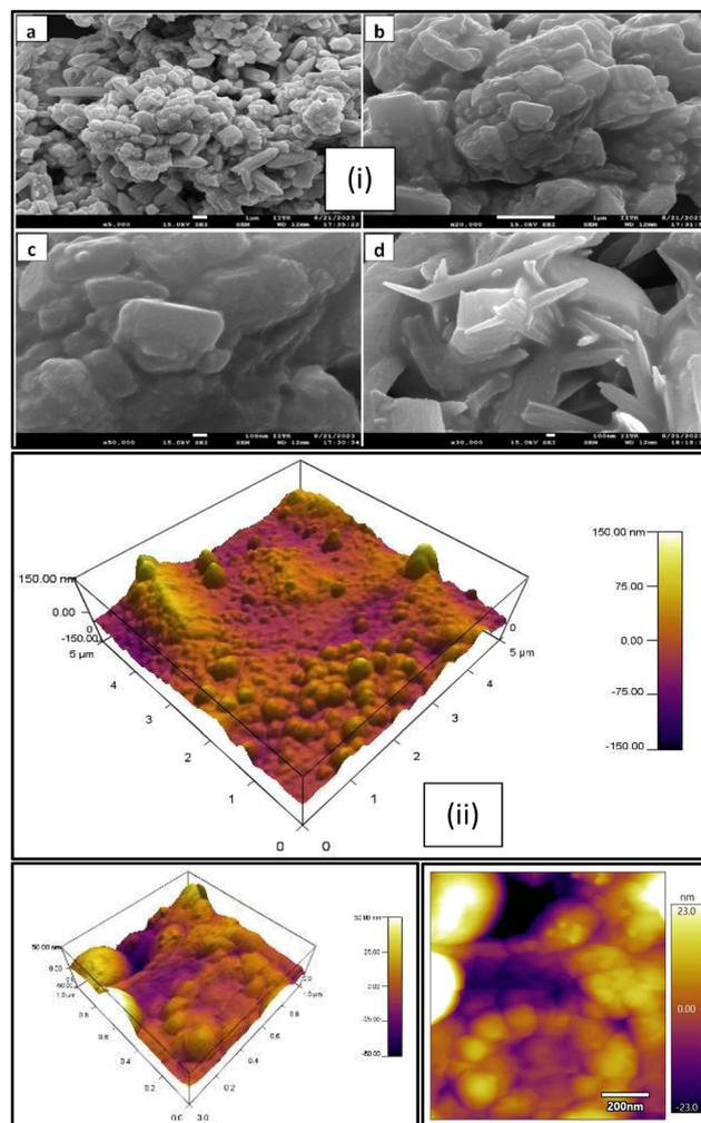
Fig. 5 (i) SEM images of the PANI/Te powder, (a, b) Scale-1 μm &amp; (c, d) Scale-100 nm and (ii) AFM images of the PANI/Te-PVA film.
