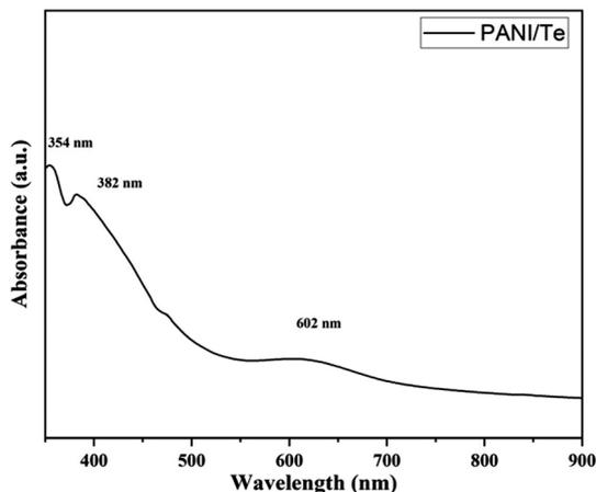
Fig. 2 UV-visible spectrum of PANI/Te in DMSO.
