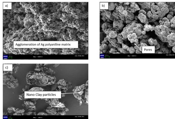
Fig. 3 SEM images of (a) Ag-PANI, (b) Ag-PANI/NC-10%, and (c) nano clay.
