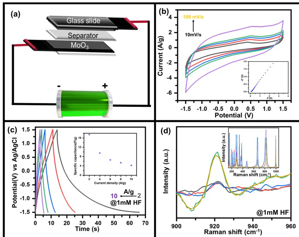
Fig. 4 (a) Schematic diagram of as-fabricated  $\text{MoO}_3//\text{AC}$  supercapacitor device, (b) CV curves measured at scan rates of 10 to  $100 \text{ mV s}^{-1}$  along with the corresponding EIS plot (ESI<sup>†</sup>), (c) GCD plots at  $2 \text{ A g}^{-1}$  to  $10 \text{ A g}^{-1}$  along with variation of specific capacitance as a function of current density (inset) and (d) *in situ* Raman spectra of asymmetric supercapacitor device during the charging and discharging process.
