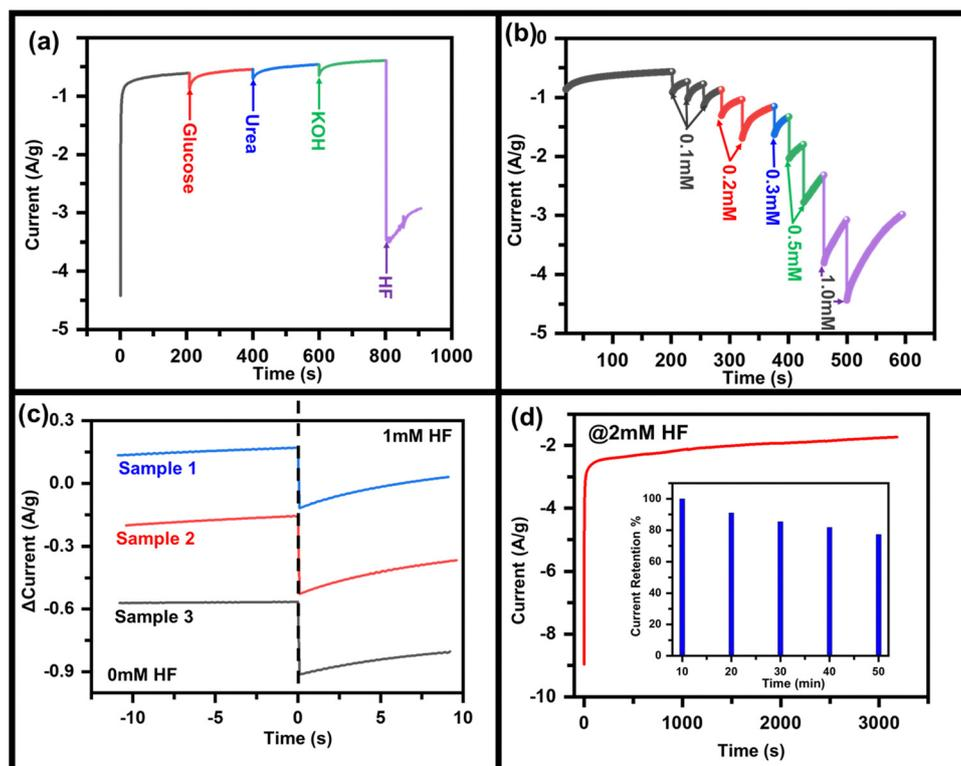
Fig. 3 Chronoamperometric response of  $\text{MoO}_3/\text{CC}$  (a) upon the addition of 1 mM HF, glucose, urea, and KOH, (b) upon the addition of different concentrations of HF (0.1, 0.2, 0.3, 0.5, and 1.0 mM). (c) Response time of the sensor for three different batches of the sample under 1 mM HF, and (d) long-term stability (inset: current retention versus time graph) test of the  $\text{MoO}_3/\text{CC}$  electrode.
