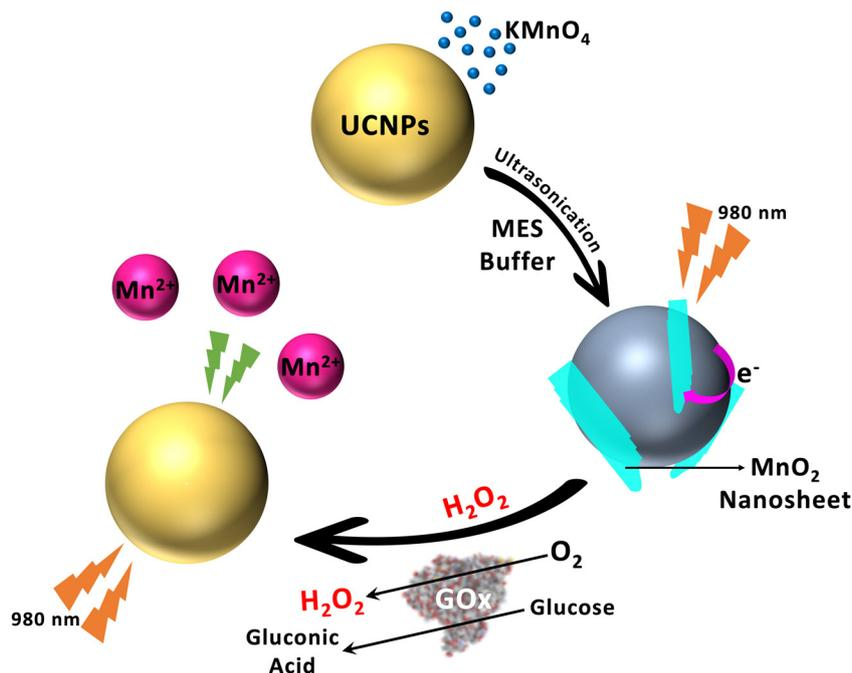
Fig. 12 The design of a H<sub>2</sub>O<sub>2</sub> and glucose detector via a MnO<sub>2</sub> NS-modified UCNP.
