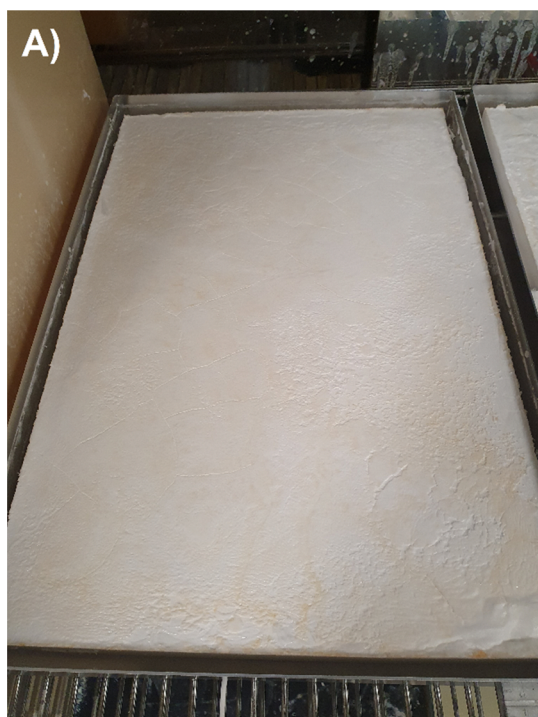
Fig. 3 (A) A 45 \times 30 \times 5 cm panel of an SRA (B) a 45 \times 60 \times 5 cm panel of the 1xSRA.
