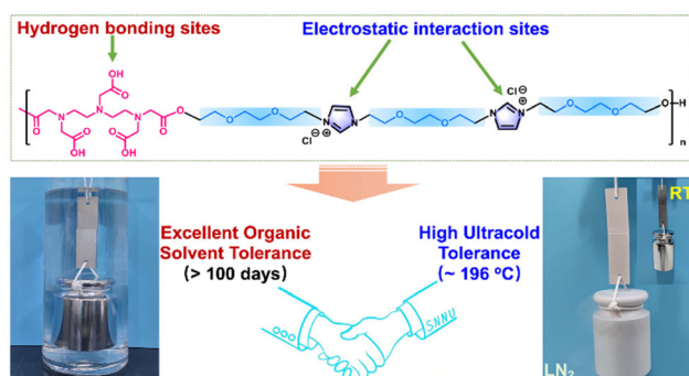
Fig. 22 The interfacial adhesion to a combination of electrostatic interactions and hydrogen bonds, obtained from Deng et al. 75 Reproduced from ref. 75 with permission from ACS, 2022.
