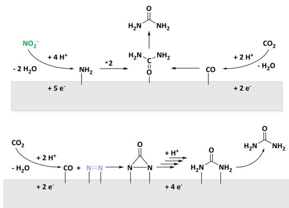
**Fig. 4** Reaction pathways of electrochemical urea synthesis via  $\text{NO}_2^-$  (top) or  $\text{N}_2$  (bottom) activation and parallel  $\text{CO}_2$  reduction to CO.
