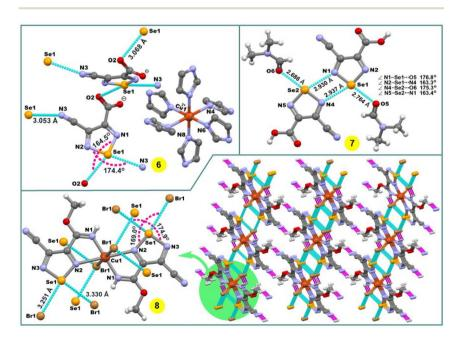
Fig. 2 Crystal structures of 6–8. H atoms in 6 are omitted for clarity. The chalcogen and hydrogen bonds are shown in light blue and pink colour, respectively.
