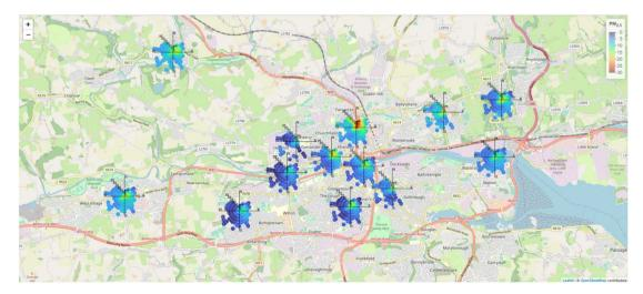
Fig. 10 Polar plots showing associations between wind speed and direction, and local PM<sub>2.5</sub> levels at the locations monitored in the sensor network.
