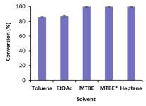
Fig. 2 Conversions for the reduction of cyclohexenone 1a catalysed by free TsOYE in organic solvents. Conditions: 10 mmol 1a, 10 U BsGDH, 20 mmol glucose, 0.2 mmol NADPH, 1.4 μmol TsOYE, organic solvent (91.7% v/v, 8.3% v/v buffer), 900 rpm, 30 °C, 24 h. \*Buffersaturated MTBE. Data are average of duplicates (see ESI† Table S2).
