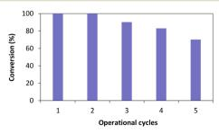
Fig. 6 Operational cycles of TsOYE immobilised on Celite R-633 for the reduction of cyclohexenone 1a in MTBE. Conditions: 50 mg TsOYE-Celite R-633, 10 mmol 1a, 1 mmol NADP<sup>+</sup>, 2 mg GDH-101, 27.7 mmol glucose, 25 mg Na<sub>2</sub>HPO<sub>4</sub>·12H<sub>2</sub>O/Na<sub>2</sub>HPO<sub>3</sub>·5H<sub>2</sub>O, MTBE (1% v/v buffer content), 1 mL volume, 900 rpm, 30 °C, 24 h each cycle.
