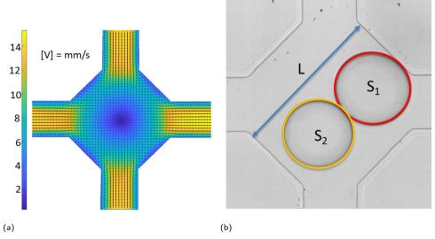
Fig. 1 Drop coalescence experiments in a microfluidic device.
