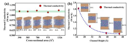
Fig. 5 (a) Thermal conductivity of water with different cross-sectional areas. (b) Thermal conductivity of water with a different channel height.
