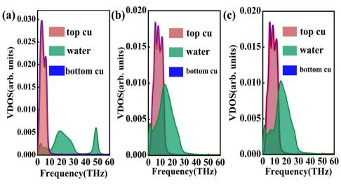
Fig. 9 The vibrational density of states of the Cu surface and water for (a) DLP, (b) LJ potential (SPC) and (c) LJ potential (TIP4P).
