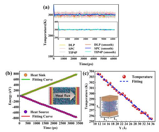
Fig. 4 (a) The temperature variation profiles of liquid water embedded in the nano-channel, (b) the cumulative energy added to the heat source and energy removed from the heat sink and heat flux across the interface is obtained by a linear fitting of the profiles, and (c) the temperature distributions of water in the nano-channel. Note that the heat flux is in units of eV ps<sup>-1</sup> and the temperature gradient is in units of K Å<sup>-1</sup>
