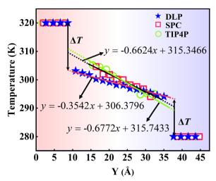
Fig. 8 The temperature distributions along the y direction calculated from dynamical simulations with DLP and empirical potentials. The x in the function expression represents the position in the y-direction, and y on behalf of temperature
