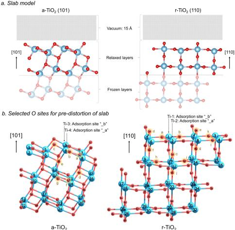
Fig. 1 Slab models used for r-TiO<sub>2</sub> (110) and a-TiO<sub>2</sub> (101) surface simulations (a) and selected O sites considered in the pre-distortion of r-TiO<sub>2</sub> (110) and a-TiO<sub>2</sub> (101) ionic structures (b). Alternative adsorption sites and number label of each atom are additionally shown
