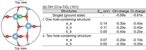
Fig. 8 Hydroxyl and chloride anions co-adsorption over r-TiO<sub>2</sub> (110) and a-TiO<sub>2</sub> (101) surfaces (a and b) and charges over hydroxyl and chloride when considering one (a.i and b.i) and two hole-containing structures (a.ii and b.ii). Computed charges in singlet (ground) state OH-,Cl-/r-TiO<sub>2</sub> (110) and OH<sup>-</sup>,Cl<sup>-</sup>/a-TiO<sub>2</sub> (101) are also given for comparison.
