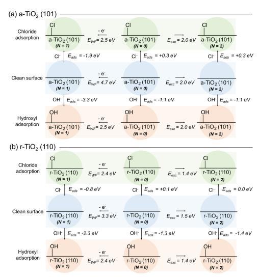
Fig. 3 Calculated adsorption energies ( $E_{ads}$ ) of hydroxyl and chloride over (a) a-TiO<sub>2</sub> (101) and (b) r-TiO<sub>2</sub> (110). Calculated work function and excitation energies ( $E_{WF}$  and  $E_{exc.}$  respectively) for each hydroxyl- and chloride-containing system are additionally shown.
