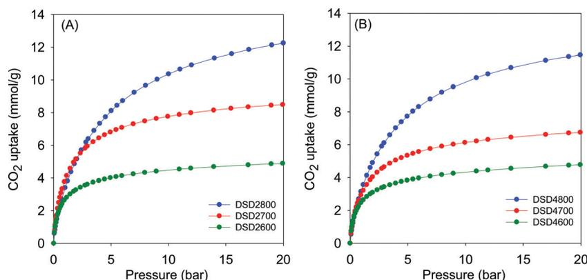
**Fig. 4** CO<sub>2</sub> uptake isotherms of carbons directly activated from sawdust (SD) at 600, 700 or 800 °C, and PO/SD ratio of 2 (A) or 4 (B).
