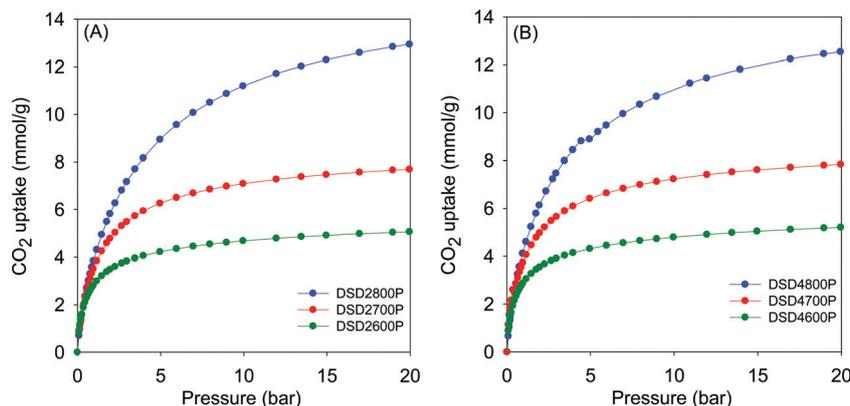
Fig. 5 CO<sub>2</sub> uptake isotherms of carbons directly compacted from sawdust (SD) at 600, 700 or 800 °C, and PO/SD ratio of 2 (A) or 4 (B).
