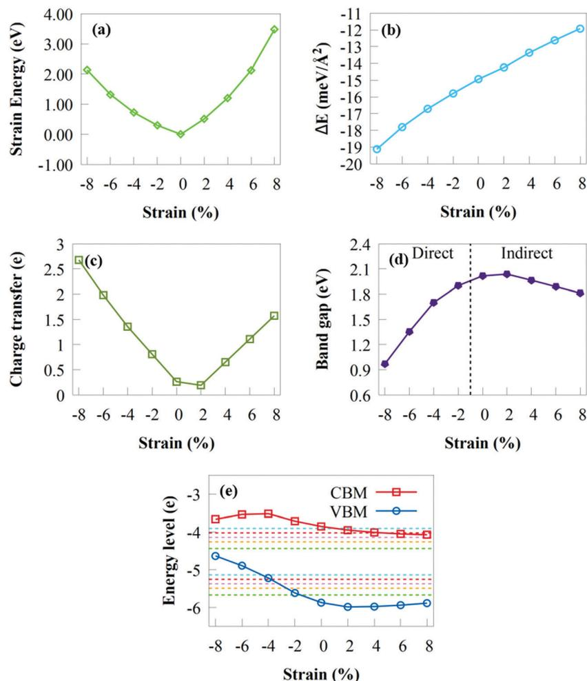
Fig. 7 (a) Strain energy, (b) binding energy, (c) charge transfer, (d) bandgap energies and (e) band edges of the  $\text{GeI}_2/\text{C}_2\text{N}$  vdW heterostructure under different biaxial strains. Green, orange, magenta, red and cyan dashed lines denote  $\text{pH} = 0, 3, 5, 7$  and  $9$ , respectively.
