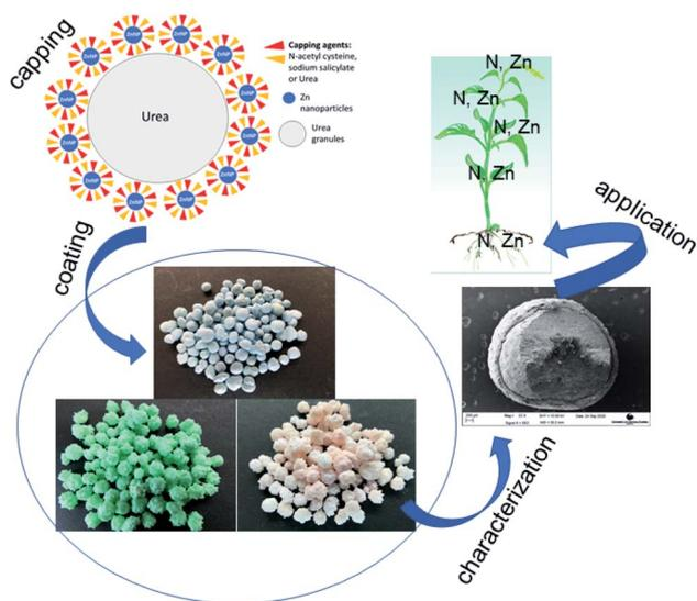
**Fig. 6** Schematic depiction of the synthesis of dual-capped Zn nanoparticles, functionalization of urea granules with the capped nano formulations, and evaluation of the nanofertilizer products in plant.
