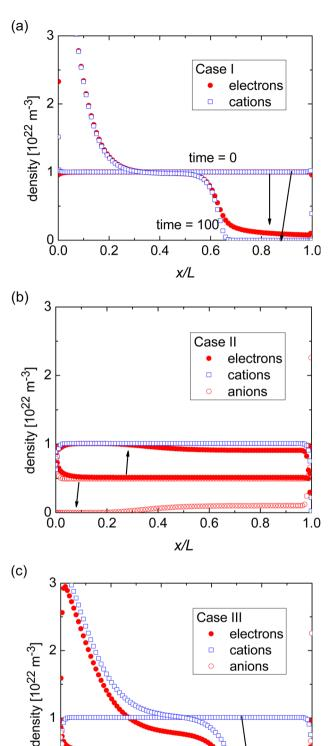
Fig. 2 Simulated profiles of the electron, cation, and anion densities for Cases I, II, and III. The arrows indicate how the density profiles change from before to after the application of the bias voltage stress.
