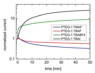
Fig. 5 Temporal response of the current in TBAF, TMAF, TBAI, and TBABF<sub>4</sub> doped devices under application of 2 V  $\mu$ m<sup>-1</sup> bias electric field.
