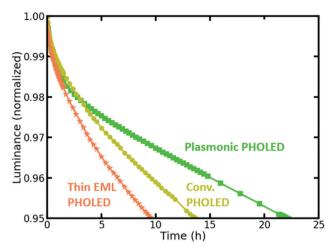
Fig. 4 Lifetime curves of the plasmonic PHOLED and reference thin and conventional EML devices aged at 80 mA cm<sup>-2</sup>.
