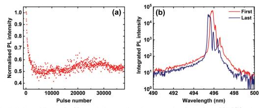
Fig. 4 Above threshold photostability data. Part (a) shows the integrated intensity versus number of pulses for the DPAVB/PS cavity at  $P = 2 P_{th}$ . Part (b) shows the first (red) and last (blue) spectra recorded, indicating that the microcavity remained in the non-linear emission regime over more than 37 000 pulses.
