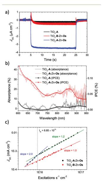
Fig. 3 (a) Amperometric i-t curves under 1 equivalent AM 1.5 solar irradiation passed through a 570 nm long pass filter (shutter open at t = 5 s, shutter closed at t = 25 s), (b) IPCE and absorptance spectra for  ${\rm TiO_2\text{-}A\text{-}Zn\text{-}Os}$  and  ${\rm TiO_2\text{-}A}$ , and (c)  $J_{\rm sc}$  with respect to excitation rate for  $TiO_2$ -**A**-Zn-**Os** and  $TiO_2$ -**B**-Zn-**Os** ( $\lambda_{ex}$  = 635 nm). All measurements were obtained at 0 V.
