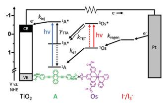
Fig. 1 Integrated TTA-UC solar cell architecture with energetics and dynamics as well as the structure of A and Os. ( $k_{inj}$  = electron injection,  $\gamma_{\text{TTA}}$  = second order rate constant for TTA,  $k_{\text{TET}}$  = triplet energy transfer,  $k_{\rm eT}$  = electron transfer, and  $k_{\rm regen}$  = regeneration rate constants)
