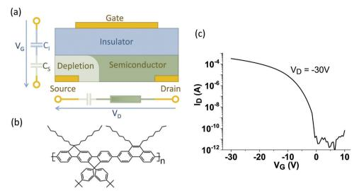
Fig. 1 (a) Schematic of bottom-contact top-gate structure used for transistors in this work. (b) Chemical structure of poly(indenofluorenephenanthrene) semiconductor. (c) Transfer characteristic of a polymer FET with near-ohmic source/drain electrodes, with channel length 5 μm, and channel width W = 1 cm.
