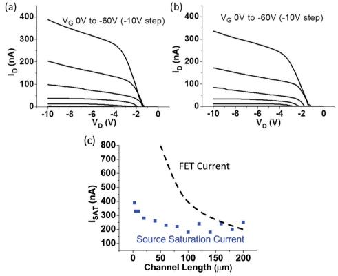
Fig. 4 (a) Examples of output characteristics of high barrier SGTs with channel lengths (a)  $L=20~\mu m$  and (b)  $L=200~\mu m$  (c) currents extracted at the onset of saturation and  $V_G=-60~V$  for transistors of different channel lengths. For this batch the gate leakage is moderate at low  $V_D$  and drops off at increasing drain voltages. For other devices in this work gate leakage is negligible (below 1 nA) and is not shown.
