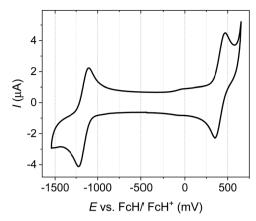
Fig. 3 Cyclic voltammogram recorded for CAT-TPE with 0.1 M  $n-Bu_4NPF_6$  in THF as the supporting electrolyte (scan rate = 100 mV s<sup>-1</sup>).
