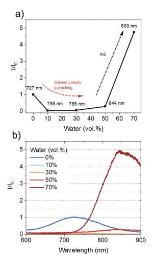
Fig. 4 (a) Intensity normalized PL spectra recorded for CAT-TPE mixtures at different vol% water ( $\lambda_{exc}$  = 400 nm); (b) plot of charge-transfer type photoluminescence intensity vs. vol% water in THF for 100 μM CAT-TPE mixtures
