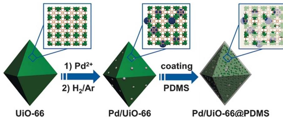
Fig. 3 Illustration of the preparation of Pd/Uio-66@PDMS. Reproduced with permission from ref. 94. Copyright (2016) Wiley-VCH.
