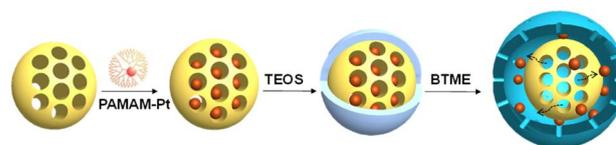
Fig. 2 Illustration of the preparation of Pt@SiO<sub>2</sub> nanoreactors through the encapsulation of PAMAM-Pt. Reproduced with permission from ref. 93. Copyright (2015) Wiley-VCH.
