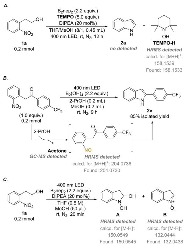
Scheme 5 Mechanistic studies. (A) Radical-quenching experiment for the synthesis of indole. (B) Annulation of *o*-nitrobenzyl ketone with an exogenous H-donor. (C) HRMS analysis of the proposed intermediates.
