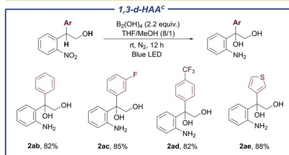
Scheme 2 Substrate scope for the synthesis of indoles and other products. <sup>a</sup>Standard conditions: 0.2 mmol scale reaction in THF/MeOH (8/1, 0.45 mL), DIPEA (0.04 mmol, 20 mol%),  $B_2nep_2$  (0.44 mmol, 2.2 equiv.), blue LED,  $N_2$ , rt, 12 h; isolated yields. <sup>b</sup> $B_2(OH)_4$  (0.44 mmol) instead of  $B_2nep_2$ . <sup>c</sup> Without the addition of DIPEA.
