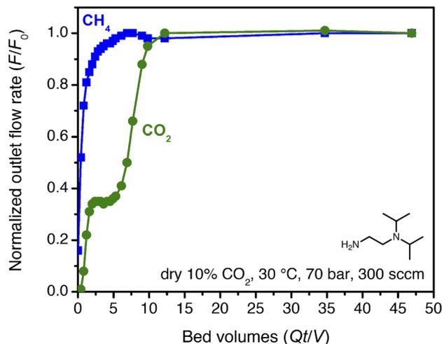
Fig. 4 Breakthrough profile for ii-2-Mg<sub>2</sub>(dobpdc) under 300 sccm of dry 10% CO<sub>2</sub> in CH<sub>4</sub> at 70 bar and 30 °C. The CO<sub>2</sub> in the initial shock corresponds to a slip concentration of 3 mol%.
