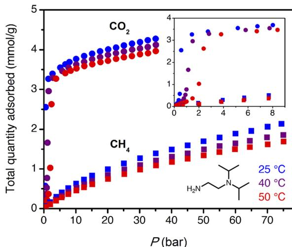
Fig. 3 High-pressure CO<sub>2</sub> (circles) and CH<sub>4</sub> (squares) adsorption isotherms for ii-2-Mg<sub>2</sub>(dobpdc) at 25 °C (blue), 40 °C (purple), and 50 °C (red). The inset shows an enlarged view of the low-pressure region.
