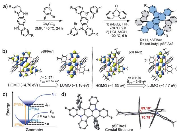
Fig. 1 (a) Synthesis procedure and structure of **pSFIac1** and **pSFIac2**. (b) The calculated distribution of HOMOs and LUMOs (isovalue = 0.03), oscillator strength ( $f$ ) and energy gap. (c) Schematic potential energy diagram of the single point energies ( $E$ ) and reorganization energy ( $\lambda$ ). (d) Single-crystal X-ray structure of **pSFIac1**. One molecule as an ORTEP drawing with a probability of ellipsoids of 50% and a side view. Hydrogen atoms are omitted for clarity.
