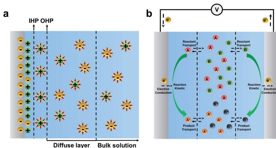
**Fig. 1** Schematic illustration for the electrochemical reactions occurring at the interface between the electrode and electrolyte. (a) Stern model of the EDL generated on a negatively charged electrode surface. (b) The key processes consist of mass transport and electron conduction in an electrochemical reaction.
