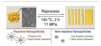
Fig. 5 Reprocessable polyhydroxyurethane network nanocomposites using silica nanoparticles with different surface functionalities as reinforcing fillers.<sup>68</sup>
