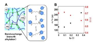
Fig. 6 (A) Schematic representation of the vitrimer-like composite with silica-nano particles. (B) Variation of  $(\langle \tau^* \rangle)$  and  $\beta$  as a function of  $\Phi_P$  (see the explanation of  $\langle \tau^* \rangle$  and  $\langle \beta \rangle$  in the main text). From ref. 71 produced/adapted by permission of Springer Nature.
