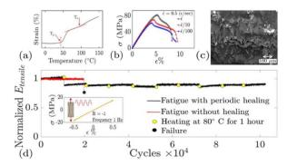
Fig. 7 Reversing fatigue damage in vitrimers by repeated doses of healing. (a) Strain measured in a dilatometric experiment with heating rate of 2.5 K min<sup>-1</sup> at stress of 25 kPa. (b) Static tensile testing at room temperature and for three different strain rates. (c) Typical fracture surface image of the failed vitrimer. (d) Fatigue test showing normalized modulus vs. the number of cycles of fatigue loading.<sup>82</sup>
