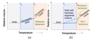
Fig. 3 Temperature dependent phase transitions of vitrimers. (a)  $T_{\rm g}$  below  $T_{\rm v}$  and (b)  $T_{\rm g}$  above  $T_{\rm v}$ .
