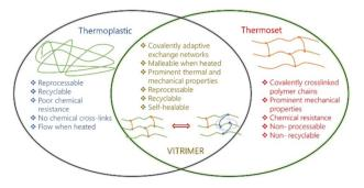
Fig. 1 Schematic representation of vitrimers' properties/advantages, compared with thermoplastic and thermoset.
