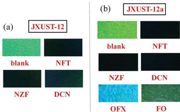
Fig. 7 Optical images of JXUST-12 (a) and JXUST-12a (b) based fluorescent test papers with various drugs under 365 nm UV light.
