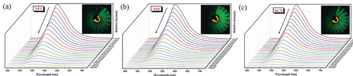
Fig. 5 Emission spectra of **JXUST-12** dispersed in EtOH solutions with various concentrations of NFT (a), NZF (b) and DCN (c). (Inset: photographs of **JXUST-12** with NFT (a, 0–200  $\mu\text{M}$ ), NZF (b, 0–170  $\mu\text{M}$ ) and DCN (c, 0–196  $\mu\text{M}$ ) under a 365 nm UV-lamp.)
