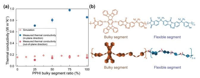
Fig. 9 (a) Relationships between the bulky segment ratio and thermal conductivity for pentiptycene-based poly(o-hydroxyimide) copolymers. Thermal conductivities are calculated by molecular dynamic simulation (MD simulation)<sup>128</sup> and experimental results for the in-plane direction and out-of-plane direction. 128 (b) Chemical structures of pentiptycene-based poly(o-hydroxyimide) copolymers and schematic of bulky and flexible segments. 128
