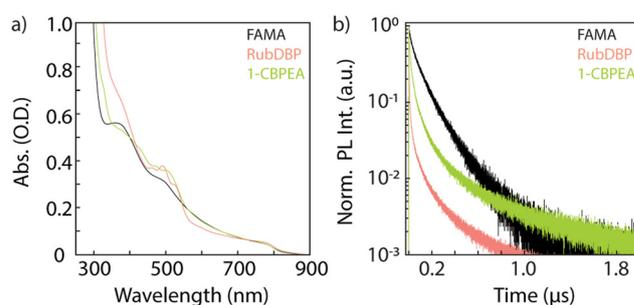
**Fig. 3** (a) Absorption spectra for the FAMA perovskite thin film (black) and bilayer devices (RubDBP: pink, 1-CBPEA: green). (b) Perovskite PL decays for the FAMA and bilayer devices under 780 nm excitation at an excitation density of  $44.2 \text{ mW cm}^{-2}$ . A 780 nm notch filter and an 800 nm long pass filter were used to remove laser scatter and isolate the perovskite emission.
