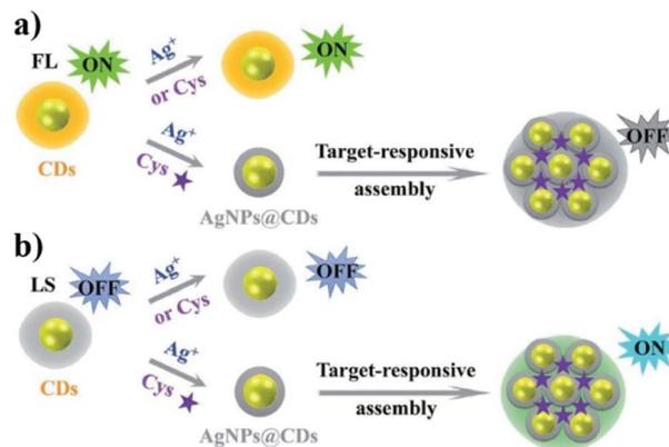
Fig. 17 Representation of CNPs for  $\text{Ag}^+$  sensing *via* (a) fluorometric and (b) light-scattering (reproduced with permission from *Anal. Methods*, 2017, 9, 5611–5617, Copyright 2017, The Royal Society of Chemistry).
