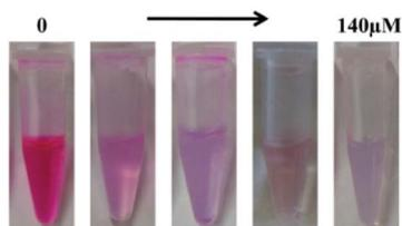
Fig. 23 Images of CNP solution for  $\text{NaClO}$  sensing upon the addition of different concentrations of  $\text{NaClO}$  (reproduced with permission from *Anal. Methods*, 2016, 8, 1157–1161, Copyright 2016, The Royal Society of Chemistry).
