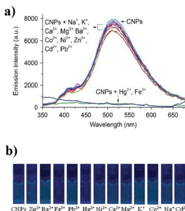
Fig. 16 (a) Emission spectra and (b) images of CNPs under a UV lamp in the presence of different cations upon excitation at 365 nm (reproduced with permission from *J. Lumin.*, 2016, 173, 243–249, Copyright 2016, Elsevier).
