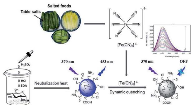
Fig. 19 Schematic representation of fluorescence enhancement and the  $\text{Fe}^{3+}$  detection process of the N-CD probe (reproduced with permission from *New J. Chem.*, 2016, 40, 10213–10218, Copyright 2016, The Royal Society of Chemistry).
