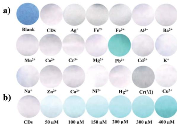
Fig. 22 Photos of strips containing CNPs and (a) different metal ions and (b) with different amounts of  $\text{Pb}^{2+}$  (reproduced with permission from *J. Mater. Chem. B*, 2019, 7, 5502, Copyright 2019, The Royal Society of Chemistry).
