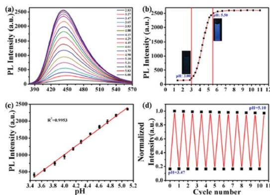
Fig. 3 (a) Fluorescence spectra at different pH values, (b) plot of the emissions during titration, (c) liner response of the CNPs to pH value, and (d) recovery test (adapted with permission from *Talanta*, 2018, 186, 80–87, Copyright 2018, Elsevier).
