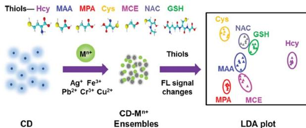
Fig. 8 Schematic representation of the fluorescent sensor array for the detection and discrimination of thiols (adapted with permission from *Sens. Actuators, B*, 2018, 266, 553–560, Copyright 2018, Science Direct).
