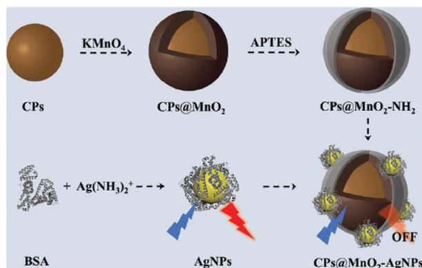
Fig. 10 Schematic representation of the synthesis of CNPs@MnO<sub>2</sub> (reproduced with permission from *Nanoscale*, 2019, 11, 18845–18853, Copyright 2019, The Royal Society of Chemistry).
