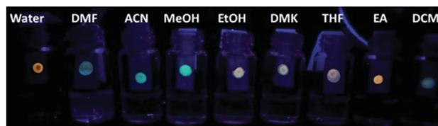
Fig. 6 Images of paper sensor strip containing CNPs after exposure to the vapor of solvents taken under a UV lamp (365 nm) (reproduced with permission from *RSC Adv.*, 2016, 6, 83501–83504, Copyright 2016, The Royal Society of Chemistry).
