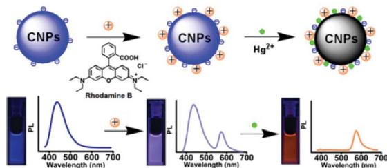
Fig. 15 Sensing mechanism of  $\text{Hg}^{2+}$  by CNPs containing RhB (reproduced with permission from *ACS Appl. Mater. Interfaces*, 2014, 6, 21270–21278, Copyright 2014, the American Chemical Society).
