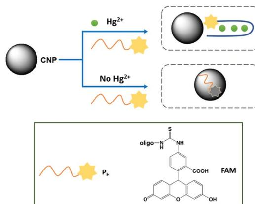
Fig. 14 Schematic representation of Hg<sup>2+</sup> sensing mechanism by CNPs based on conformational change of DNA strand.
