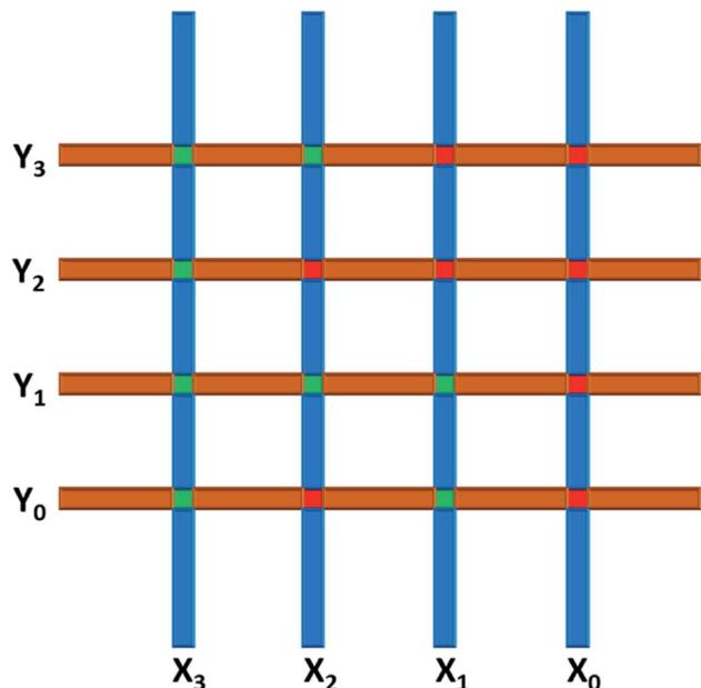
Fig. 16 A  $4 \times 4$  crossbar storage structure (red – “0”; green – “1”).
