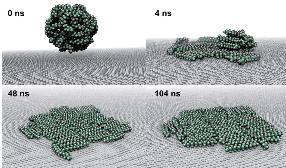
Fig. 6 Formation of a pentadecane monolayer at the graphene–water interface. (A) Initially a droplet of pentadecane was placed above the graphene–water interface. (B–D) A partially ordered monolayer is formed within a few nanoseconds.
