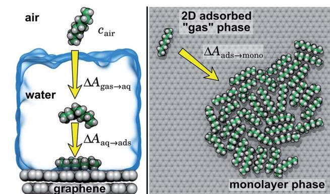
Fig. 3 Diagram of free-energy changes for adsorption of alkanes to the graphene–water interface from air.  $\Delta A_{\text{gas} \rightarrow \text{aq}}$  is the hydration free energy.  $\Delta A_{\text{aq} \rightarrow \text{ads}}$  is the free energy for single-molecule adsorption from the aqueous phase to the graphene–water interface.  $\Delta A_{\text{ads} \rightarrow \text{mono}}$  is the free energy for condensing from the 2D gas phase to the bulk of the monolayer condensed phase.
