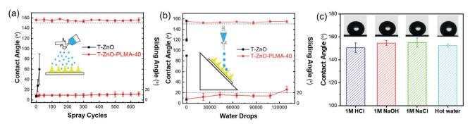
Fig. 6 The durability of T-ZnO coated mesh and T-ZnO/PLMA-40 against (a) water spray impact and (b) water droplet impact. (c) Contact angles of strong acid, base, salt solution, and 70 °C water droplets on T-ZnO/PLMA-40.
