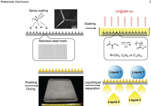
Fig. 1 Schematic representation of the preparation of T-ZnO/polymer hybrid-coated mesh through ZnO-initiated photopolymerization, and its application for liquid/liquid separation. A fully coated 25 cm  $\times$  25 cm mesh is shown as an example in the photo.
