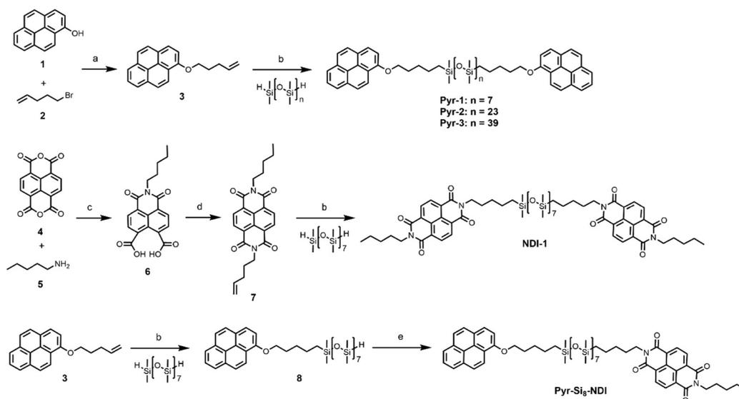
**Scheme 1** Synthesis of pyrene and NDI blocks and the corresponding **Pyr-1**, **Pyr-2**, **Pyr-3**, **NDI-1** and **Pyr-Si<sub>8</sub>-NDI**. Reaction conditions: (a)  $K_2CO_3$ , DMF, 80 °C, 24 h (89%); (b) Karstedt's catalyst, DCM, 1–2 h (51–83%); (c) DMF, microwave (i) 75 °C, 5 min, (ii) 140 °C, 15 min (22%); (d) 4-pentene-1-amine, DMF, microwave (i) 75 °C, 5 min, (ii) 140 °C, 15 min (48%); (e) NDI **7**, Karstedt's catalyst, DCM, 4 h (45%).
