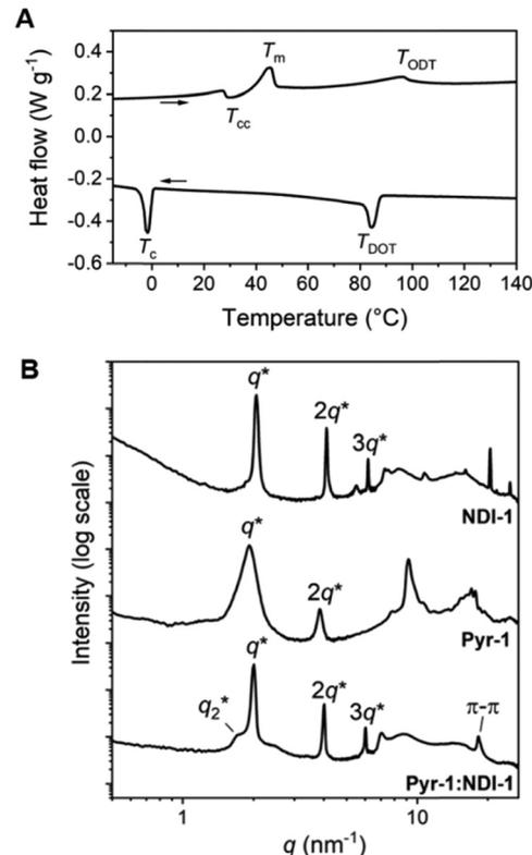
Fig. 1 (A) DSC trace (second heating and cooling cycle) of **Pyr-1:NDI-1**. A temperature ramp of 10 K min<sup>-1</sup> was used. Endothermic heat flows have a positive value. (B) 1D transmission scattering profiles of **Pyr-1:NDI-1** (bottom), **Pyr-1** (middle) and **NDI-1** (top) at room temperature.
